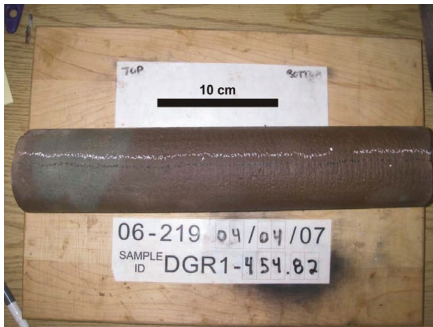
Figure 2.29: Core Sample of Green and Red Calcareous Shale, Upper Ordovician Queenston Formation, 454.82 mBGS, DGR-1
