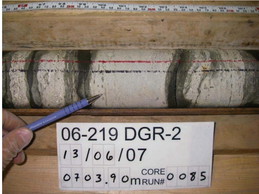
Figure 2.26: Core Sample of Argillaceous Limestone and Shale Interbeds, Sherman Fall Formation, 703.90 mBGS, DGR-2
